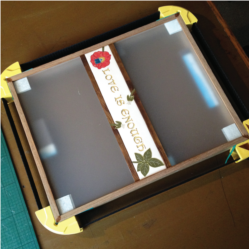
Figure 20: Constructing the teak wood box to encapsulate a frosted acrylic lid.
